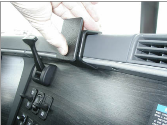
3. Press firmly forward on the lower part of the ProClip so the angled edge snaps into the gap between the center panel and the dashboard edge.
