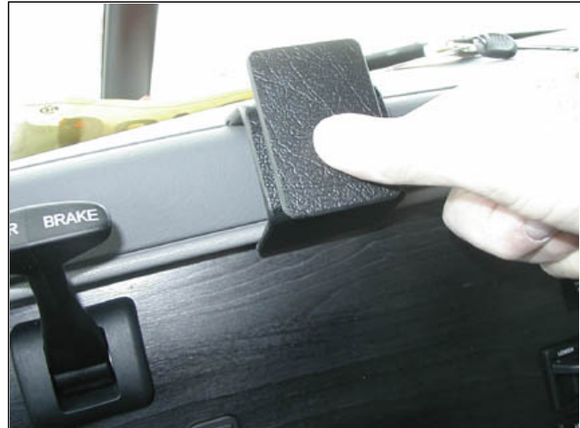
2. Place your index finger behind the lower part of the ProClip and pull down so the angled edge snaps over the dashboard edge.
