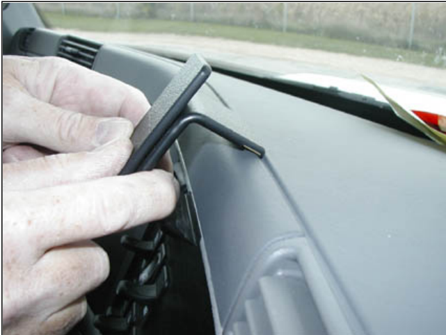
1. Peel off the cover of the adhesive tape on the ProClip. Place the angled edges on the upper part of the ProClip into the groove in the dashboard.
